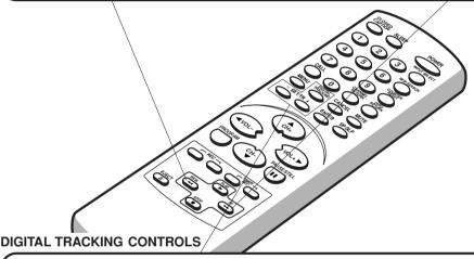
When a tape is played, the Digital Auto Tracking system automatically adjusts the tracking to obtain the best possible picture. If noise bars appear during playback, adjust the tracking manually as follows:
